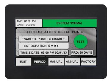
The colour touchscreen display on the Intellistat TS provides all electrical parameters, inverter status, programmable inverter, battery testing, and data-logging. Optional NetMinder™ communications allow remote monitoring and reporting via BACnet/IP or BACnet MS/TP, Ethernet TCP/IP, MODBUS TCP, or MODBUS RS485.
