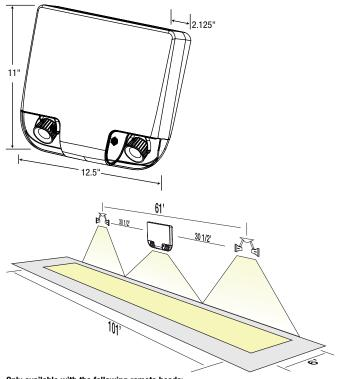
Only available with the following remote heads: S1-06V4LR / S2-06V4LR M1-06V4LR / M2-06V4LR
