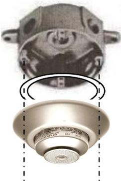
The detector is installed using rain-tight conduit and a standard, approved weatherproof electrical enclosure as shown above. A neoprene (or similar gasket supplied with the back box), is installed between the detector's seal plate and the back box. The wire leads are connected to the initiating circuit inside the enclosure. Unused threaded openings are sealed with threaded plugs. A decorative anodized aluminum cover ring snaps over the detector to complete the installation.
