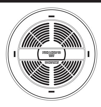
The American Sensors ESA5011, 120 Volt hardwire smoke alarm with built-in relay is an all purpose smoke alarm incorporating "dual-ionization" technology for sensing visible and invisible particles of combustion. The built-in relay allows auxiliary devices to be signalled in an alarm condition, and the unit and contacts will automatically reset upon conclusion. Up to 18 units can be interconnected for simultaneous warnings.
